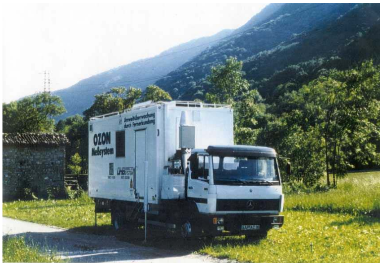
Figure 1: The mobile ozone lidar of IMK-IFU during the VOTALP Milano Experiment (Barni, Prov. di Como, 620 m a.s.l.)
